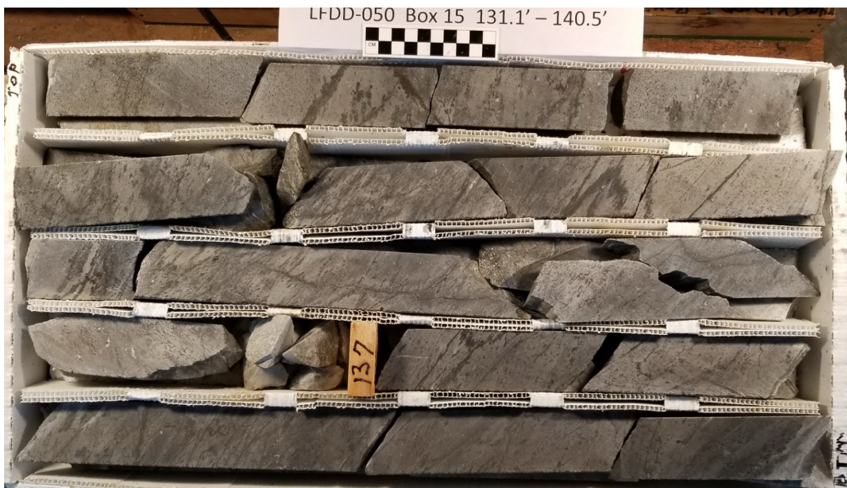
Figure 3: 2021 drill core from Loflin displaying a phyllic altered and deformed volcanoclastic. Note that the core block measurement is in feet.
