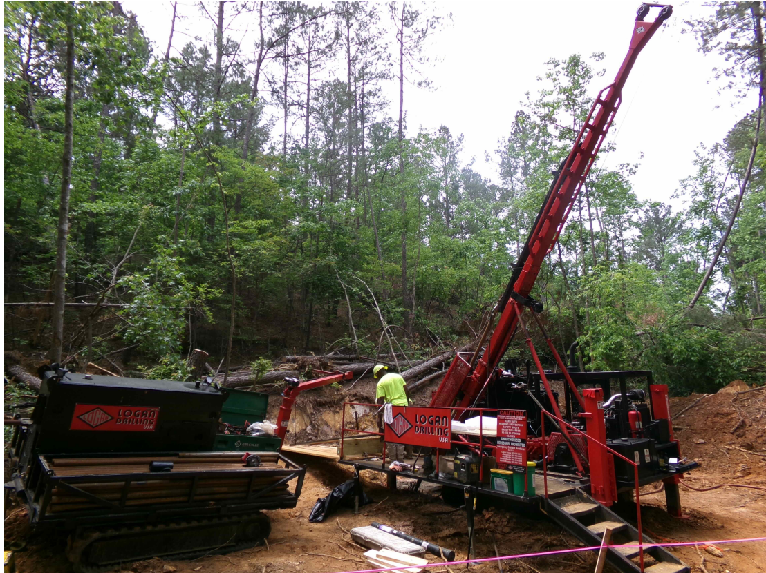
Figure 1. Setting up of the diamond drill rig at Jennings-Pioneer for the commencing of drilling
