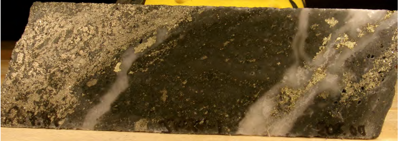
Figure 3: 0.18m segment of polished half NQ core from hole JP24-1 207.82m to 208.00m displaying Footwall Zone sulphides and veining.
