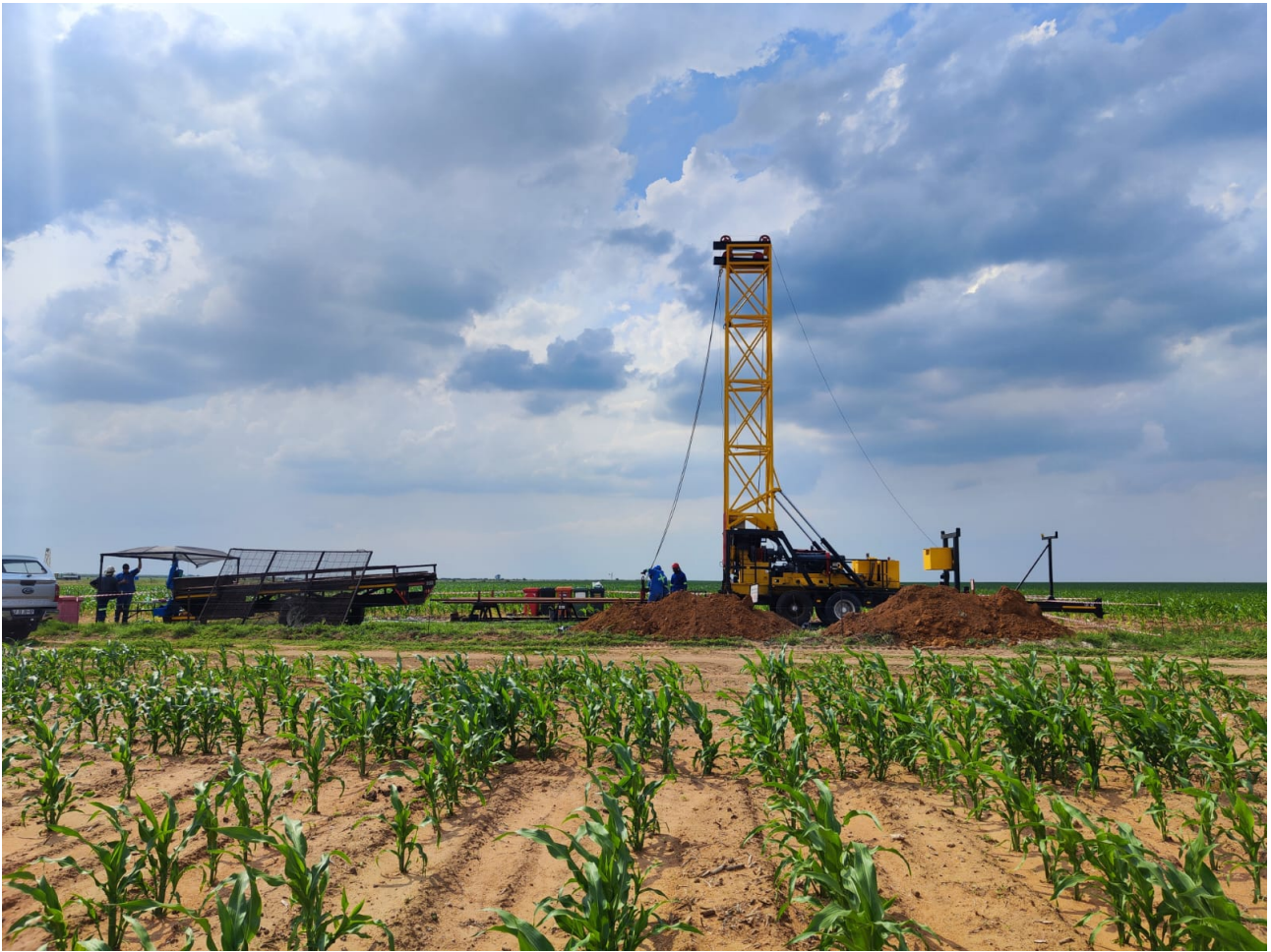
Figure 1: Diamond drilling underway at the Bothaville Project in the Witwatersrand Gold Basin
