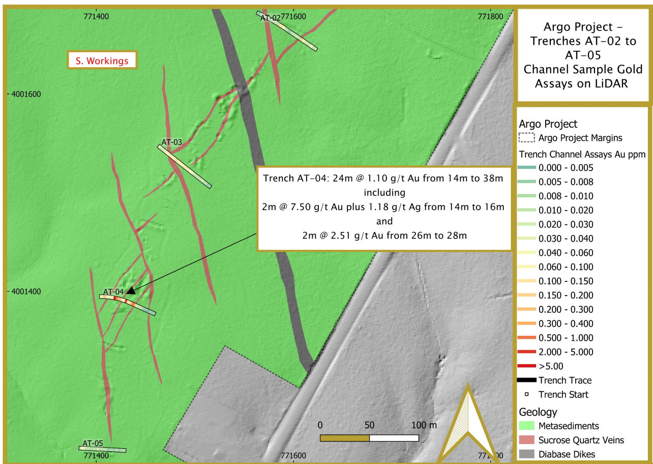
Figure 5: Plan view of trench channel sample gold assays with geology and LiDAR on the Southern Workings at the Argo Project.
