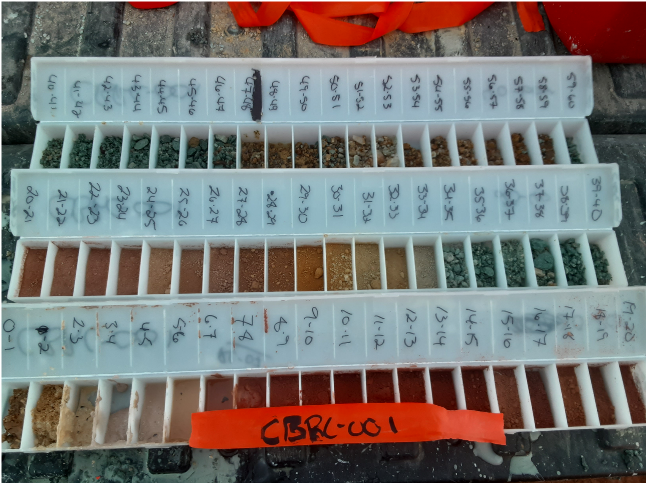
Figure 2: RC drill chips with quartz veins and alteration zones
